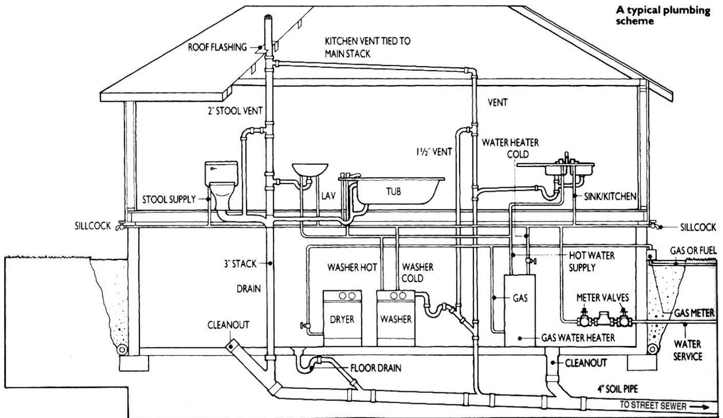
Most newer water lines are made of **copper**, and seldom become obstructed. The only time you will usually need to deal with copper pipe is when you are changing a valve or re-routing a water line. Lengths of copper pipe are soldered together, although you can use **compression fittings** – a more expensive option – to join them if you don't want to use a propane torch.
