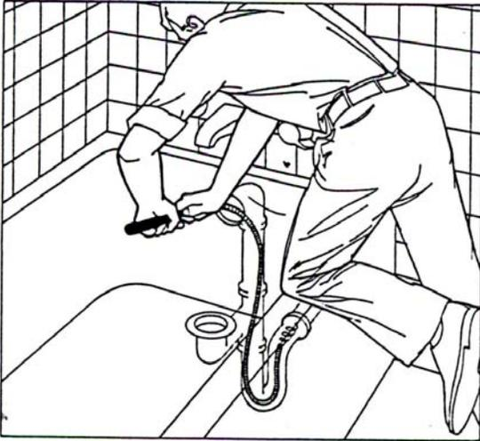
*To snake a bathtub with a hand-powered auger or electric drain snake, run the cable through the tub overflow opening to reach the P trap.*
