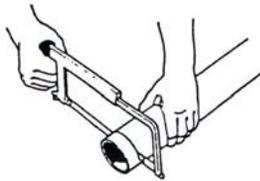
1. *Cut the pipe squarely with a hacksaw, power miter saw, or PVC tubing cutter.*
