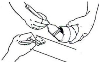
3. *Apply primer to the inside of the pipe and the outside of the fitting, and allow to dry for a few minutes. Then, brush on the PVC cement.*
