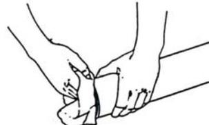
2. *Remove burrs along the cut end – both inside and outside – with a utility knife or sandpaper.*
