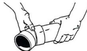
4. *Insert the pipe into the fitting as far as it will go, making sure the pieces are aligned properly, and hold for a few moments. The cement will dry quickly, so you will have little room for error.*
