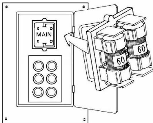
Every house should have an **ELECTRIC SERVICE PANEL** with a **MAIN SHUTOFF**, whether circuit breakers or fuses are used (cartridge main box with 6 circuits shown). The number of circuits will vary with the electrical loads in the house.
