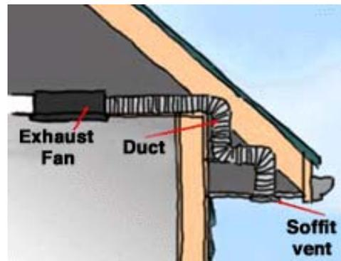
If you can't run the duct to a soffit, the project will be a bit more complicated. You can install a vent through the roof, with a special cap that includes a damper.
