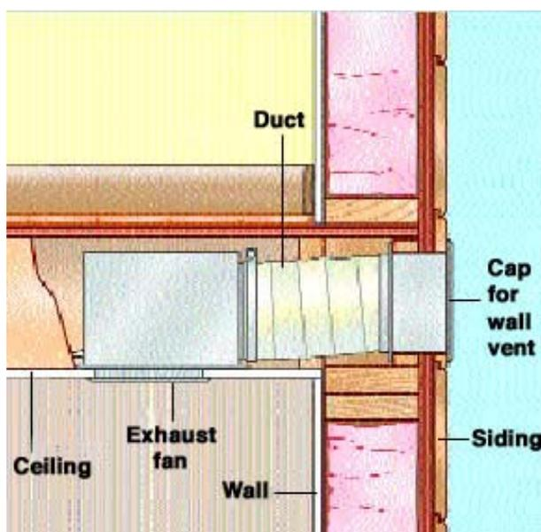
Another option is to vent the water vapor through the wall. There are even fans designed to mount on the bathroom wall, instead of the ceiling, and vent directly to the outside through hinged dampers similar to those used for clothes dryers.
