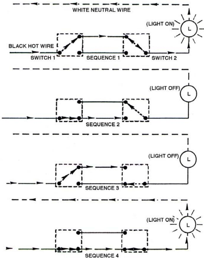
**Three-Way Switch Schematic**
