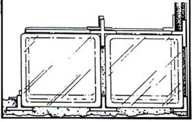
Once the panel has been assembled and the joints tooled, allow the mortar to set for another 15 - 30 minutes. Then, clean off any excess mortar from both sides of the panel and fill in any voids in the joints. If you used spacers, break off the projecting ends, leaving the body of each spacer imbedded in the mortar. After you have done all this, clean off any remaining mortar from the face of the bricks and let the panel set overnight for the mortar to harden.
