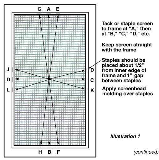
Once the screen is attached all around, apply new screen bead to the joint between the screen and the frame. (It's unlikely you'll be able to re-use old screen bead, unless extreme care is used in its removal.) The screen bead should be painted on all sides before it is applied to the screen. Trim the excess screening with a sharp utility knife. Make sure the screen bead is solid and tight into the corners.
