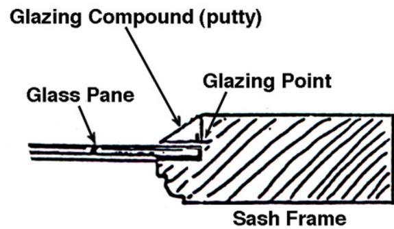
Once the glass is secure, form another snake of glazing compound as before. Push this snake into the area where the glass meets the frame on the outside. Run a glazing tool or putty knife held at a 45° angle along the edge, as described above, so that you end up with a smooth wedge of glazing compound that is not visible from inside the window.
