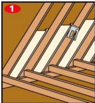
Start your job by installing baffles in areas where you need to hold back insulation. Where joists intersect with roof rafters, insert a plastic or polystyrene baffle in each rafter bay. Staple the baffles into position (*Figure 1*).
